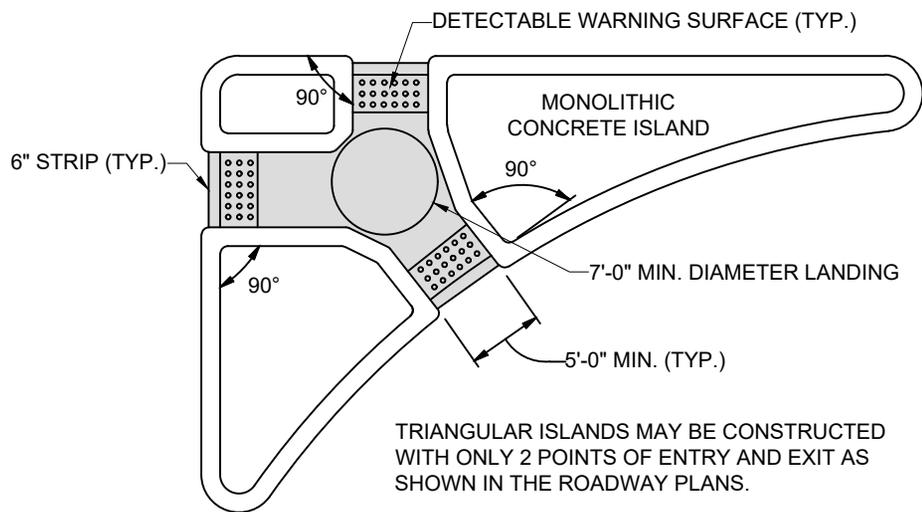
TRIANGULAR ISLANDS MAY BE CONSTRUCTED WITH ONLY 2 POINTS OF ENTRY AND EXIT AS SHOWN IN THE ROADWAY PLANS.
