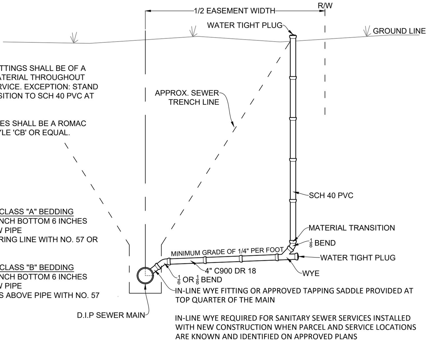
IN-LINE WYE REQUIRED FOR SANITARY SEWER SERVICES INSTALLED WITH NEW CONSTRUCTION WHEN PARCEL AND SERVICE LOCATIONS ARE KNOWN AND IDENTIFIED ON APPROVED PLANS
