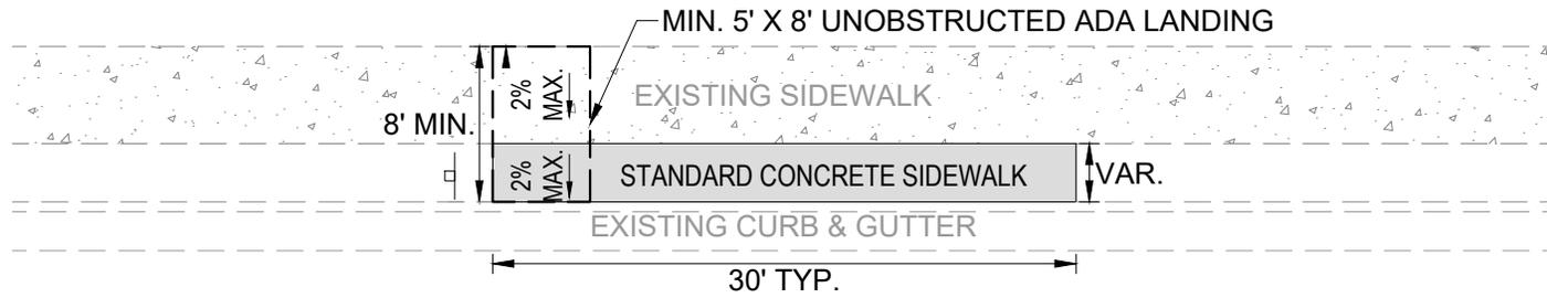
LANDING PAD W/ SIDEWALK AT BACK OF CURB
